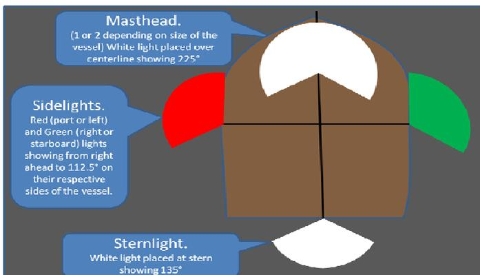
Rule 21 provides the definitions for the masthead light, sidelights, sternlight, towing light, all-round lights or task lights, and flashing or special flashing lights. Task lights are those lights which place the vessel in a special condition (e.g., all-round red over white over red for a vessel with restricted maneuverability).
