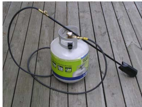
Weed-burner Propane Tank Rig
